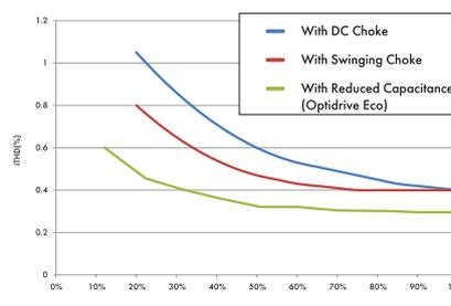
It can be clearly seen that the reduced DC link capacitance significantly reduces the total harmonic distortion at full load, and has a much greater benefit at part load compared to a conventional DC choke or swinging choke. This results in reduced overall input current and reduced transformer heating effect.
