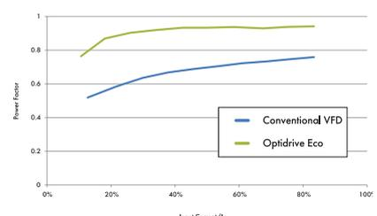
Optidrive Eco offers improved power factor over conventional VFDs under all loads.
